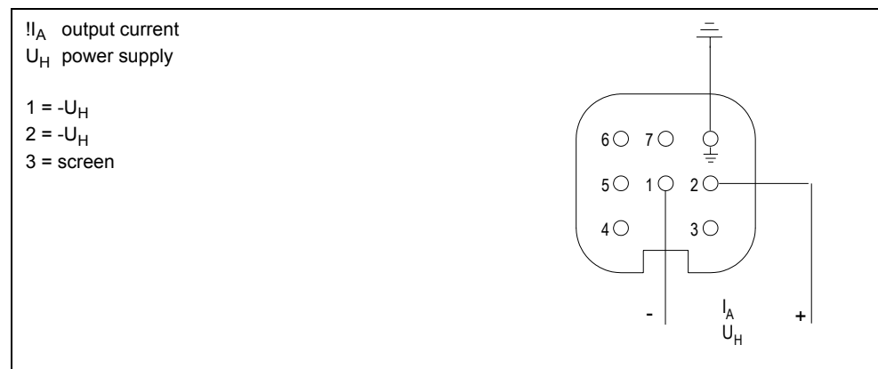
Figure 52 Connect with plug (Han 7D / Han 8U)
