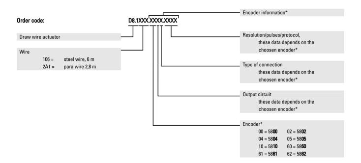
\*The type of encoder and its features the are specified.
